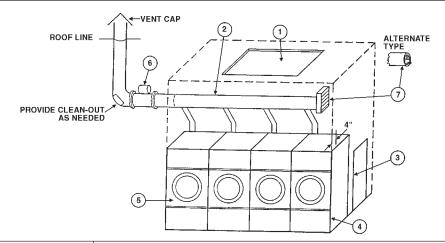
DRYER INSTALLATION WITH MULTIPLE EXHAUST For Exhaust Duct more than 14 feet (5 m) and 2 elbows equivalent and more than 0.3 inches (8 mm) static pressure.
