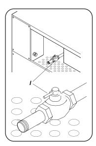
The gas supply pipe should be connected to the gas tap (I), which is on the right next to the wiring box on the back.
